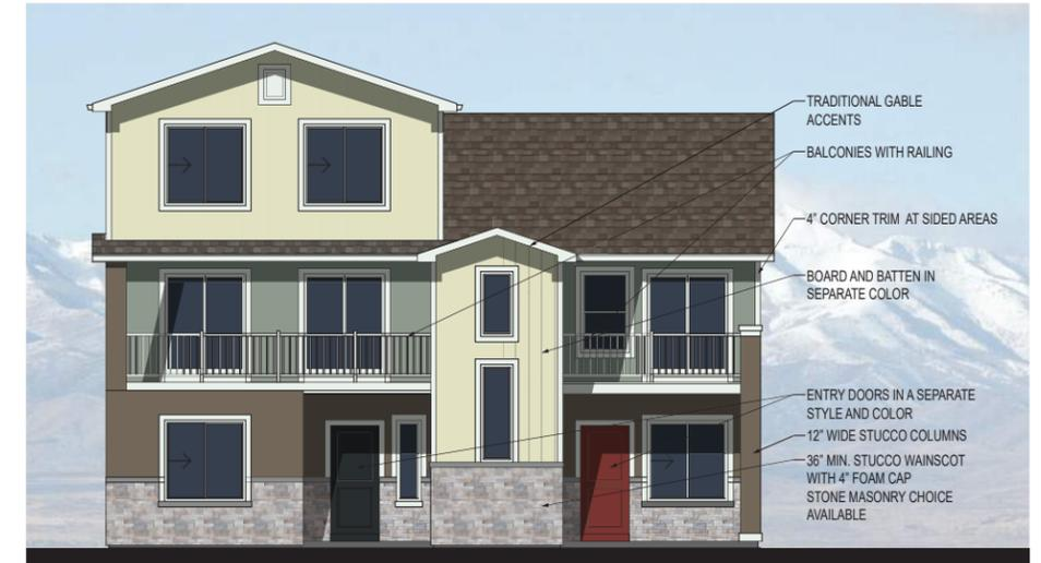
4 Typical Front Elevation - Stone Masonry Choice
