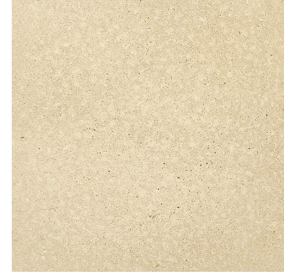
White precast concrete trim
